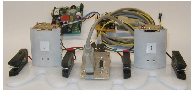
Figure 5: Charging station with two docking bays
